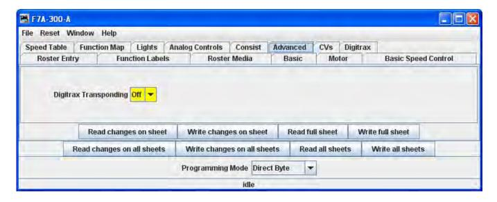
Complex Advanced pane for Tsunami OEM of the FP-45 decoder.
