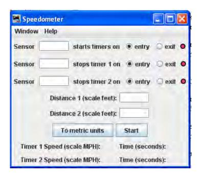
Three sensors are installed on your layout, sensor 1 and 2 for slow speeds, and sensor 1 and 3 used for higher speeds. The time to travel between the sensors is used with the distance to calculate the speed in English or Metric units
