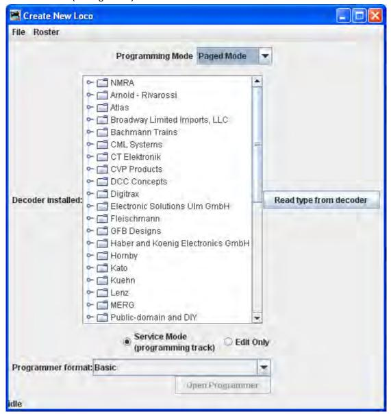
As in the screen below several possible decoders will probably be highlighted. This happens because the decoders are electrically the same but are packaged differently to fit the locomotives that they are used in. If you know which decoder is in use, then select that one. If not, in most cases any of the highlighted decoders will work, and you should select the one with the least letters at the end, since letters are often used to denote locomotive specific variations.
