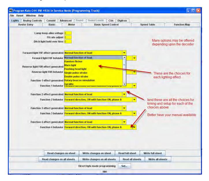
Sound decoders such as the Tsunami in our OEM FP-45 has an extremely complicated Lighting progam pane.
