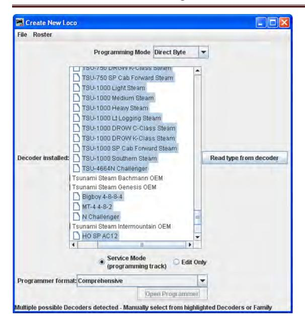
Note that we have selected a decoder, which is highlighted. Also the **Open Programmer** button is activated to allow us to enter the programmer and the Programmer format may be set to **Basic** or **Comprehensive** using drop down list.. As a beginner you may select **Basic**, or if experienced select **Comprehensive**.
