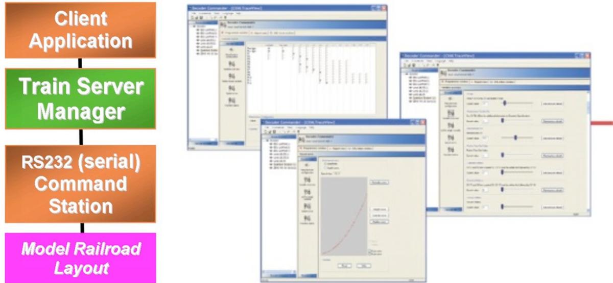
Decoder Commander is an application that runs on your desktop or laptop PC. The desktop or laptop PC is connected to a layout using a command station interface. The interface is usually a serial interface or USB device.
